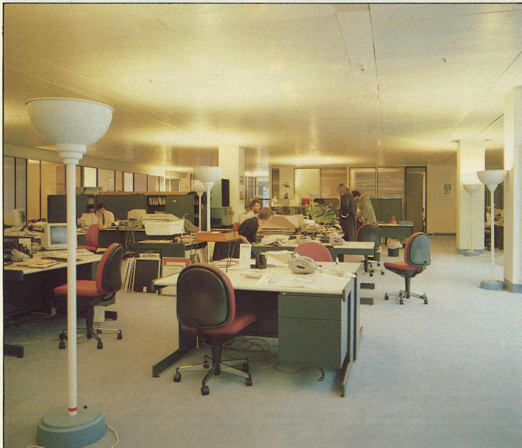
Open plan office area lit by high pressure sodium uplights.
